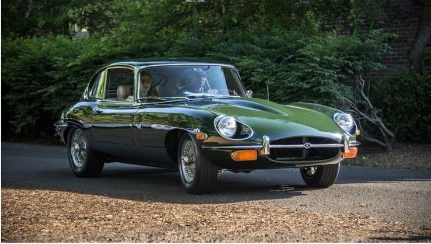
The Series II E-Type debuted in 1968 after a short run of transitional cars known as Series 1.5 in 1967 and 1968. Series II cars dropped the glass headlights while gaining a larger grille opening, and receiving restyled front and rear bumpers and fascia's. Side indicators became larger and moved to just below the front bumpers, in contrast to the slimmer side indicators that sat immediately below the headlights on the Series I cars.
